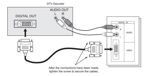
1) Connect the DTV DIGITAL RGB OUTPUT TERMINAL to the DIGITAL INPUT TERMINAL of
